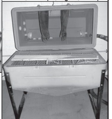
Polymer Clam Shell Cabinet Sandblaster 28"x48" work area
