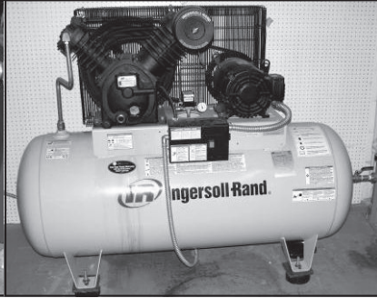
Ingersoll-Rand Air Comp T30 2545 2 stg, 10hp, 35cfm, 120gal, 220 3ph
