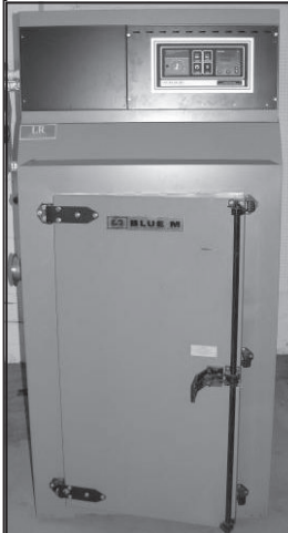
Blue M Indstrl Oven int. 24" w x 24" d x 48" h st. steel, ext. 52x40x84 208/240 3ph, 600 deg f
