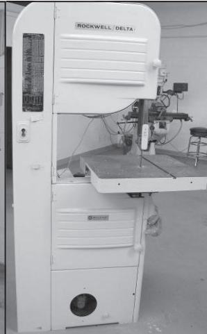
Rockwell Delta Vert. Saw 19.5" throat, 12" h, 220 3ph
