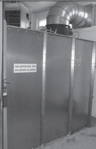
Col-Met Ind. Spray Booth 6' w x 5' d x 7' h, 4 tube light open front, 24" tube axial exhst fan, 18ga galv const
